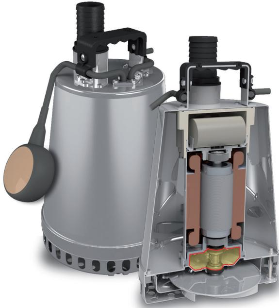
Drainage pump in 304SS, complete with twin mechanical seals in oil bath and through motor cooling which guarantees motor cooling even at low pumping levels. Strainer base can be converted to allow pumping down to 5mm for special applications.
